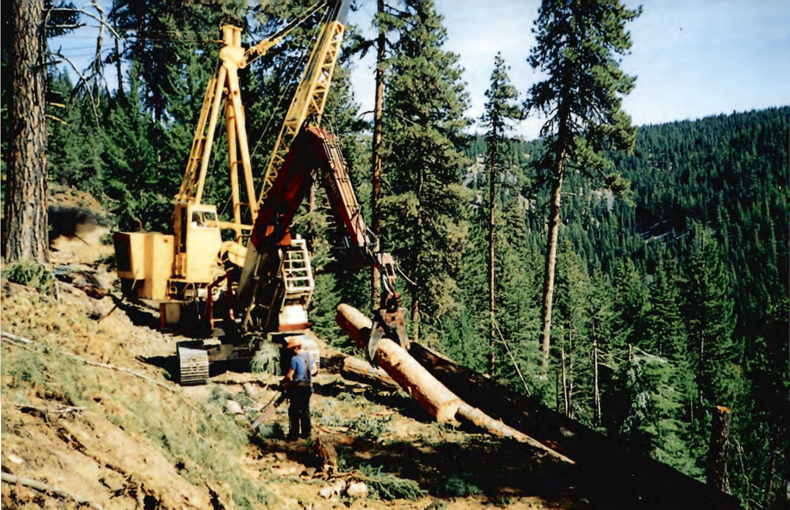
Foto 1. Cable-yarding i Yakima Indian Reservation Territory. Cable-yarding er et langt mere skånsomt transportsystem på stejle arealer, hvor erosionsfaren er stor.
